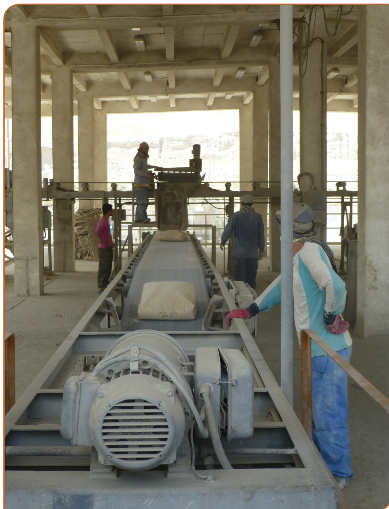
Below - Figure 5: The packhouse at the Ghori I plant can package 4000 50kg bags in seven hours with a four-headed packer. The room is extremely dusty, posing a threat to employee health and the environment.
